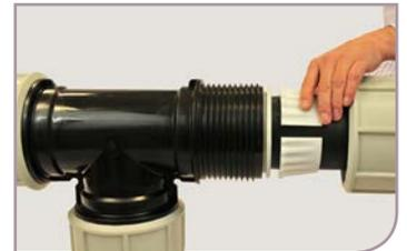
Open the white split ring and mount onto pipe with larger side against the collar ensuring that both parts meet tightly onto the fitting using a Plasson wrench.
