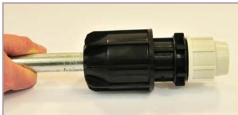
Slide the universal end of the fitting onto the pipe end until it reaches the internal fins and a resistant point is felt. **NOTE:** Do NOT force pipe end past the internal fins as this may impair joint.
