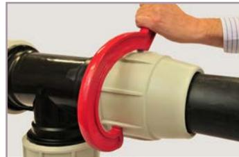
Tighten the nut with a Plasson wrench until the O-ring and collars enter the fitting and reach their end position. Unscrew nut from fitting.
