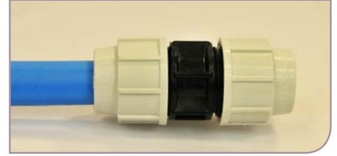
Tighten nut firmly: Hand tight on pipe 20mm (1/2") - 32mm (1"), on pipe 40mm (1 1/4") and above use a Plasson wrench.
