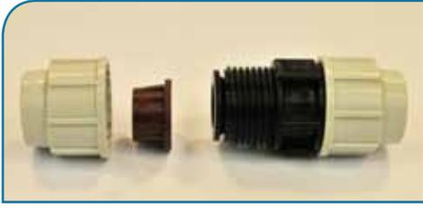
Remove nut from fitting and discard white split ring (except 35, 42, and 54mm copper, where the white split ring is used as a spacer). Push black rubber seal into fitting body and assemble components in the order shown above.
