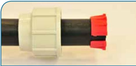
Remove nut from fitting and discard white split ring (unless using 1 1/2" pipe). Mount nut on pipe and assemble red split ring flush with the pipe end (reuse white split ring for 1 1/2" pipe).
