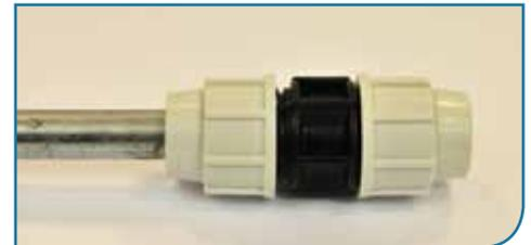
Push pipe into the body of the fitting and tighten firmly with a Plasson wrench (it is important that the pipe is NOT pushed fully up to the stop inside the fitting).
