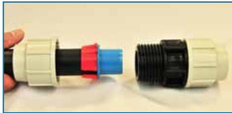
Push the barbed end of the adaptor into the pipe until it meets the stop. Then push the plain end of the adaptor into the fitting until it meets the stop.
