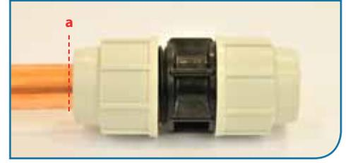
Push and twist the pipe through the nut, adaptor and metal ring into the body of the fitting, until the mark is in line with the end of the nut as shown. Tighten the nut with a Plasson wrench.
