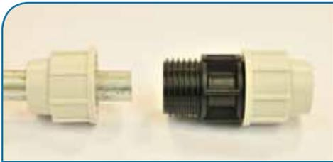
Prepare pipe by ensuring that the end is free from grease and roughen outer surface with wire wool or similar. Remove nut from end of fitting and mount onto pipe, discard white split ring.
