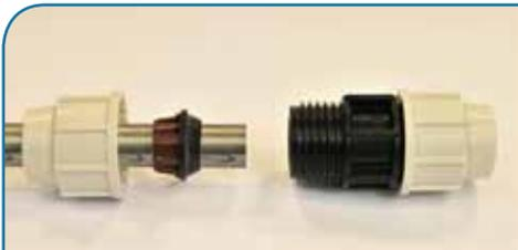
Remove nut from fitting and discard white split ring. Mount nut onto pipe followed by brown split ring and seal ring.
