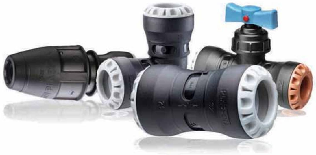
Plasson pushfit is a range of innovative push-fit fittings that provide connectivity of Polyethylene (MDPE) pipe to a variety of plumbing pipe materials. Inserting the pipe up to the fitting stop creates both seal and grip on the pipe.
